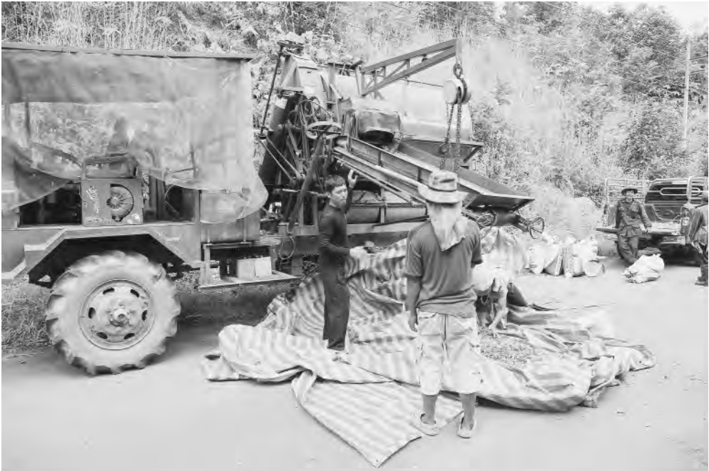
Figure 6. Mobile thresher in operation. Mae Tho Tai Village.
